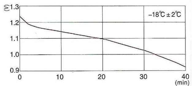
1IA discharge curve of high discharge rate Ni-cd battery at low temperature
